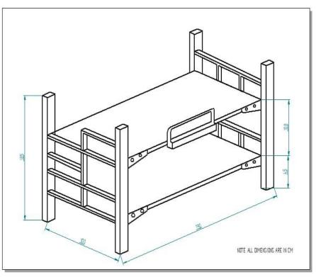
Bunk Bed Dimensions Total Height: 1.85 Mtr Total width: 1 Mtr Bunk Bed In between Gap: 1.00 Mtr Bunk Bed Metal Sheet Length & Width: Length: 1.90 Mtr Width: 1.00 Mtr Guage of Sheet : 14g
